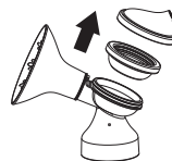
Separate the membrane lid and the membrane from the connector
