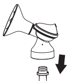
Pull the membrane out of the connector
