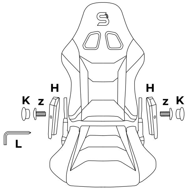
**EN:** Assemble the covers **(H)** to the metal brackets using small screws **(z)**. Use the plug buttons **(K)** to hide screw holes.
