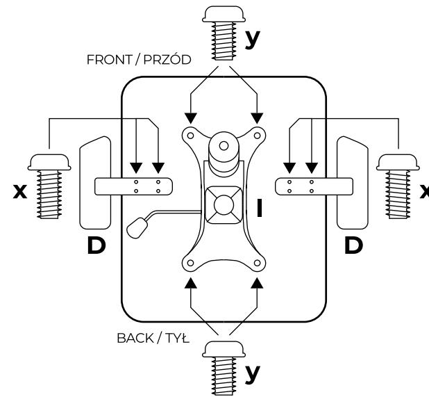
**EN:** Using M8x16mm screws **(y)**, assemble the mechanism **(I)** to the seat as shown. Then assemble the armrests **(D)** to the seat using M8x20mm screws **(x)**.
