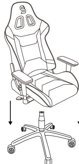
**EN:** Insert top of the gas lift into to the mounting hole of the mechanism under the seat (you may need help of another person). Push the seat down firmly.
