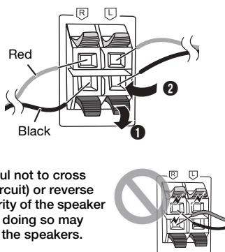
Be careful not to cross (short-circuit) or reverse the polarity of the speaker wires as doing so may damage the speakers.
