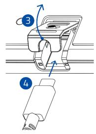
3. Push down the cable security clasp, slide it inwards, and lock it in place.
