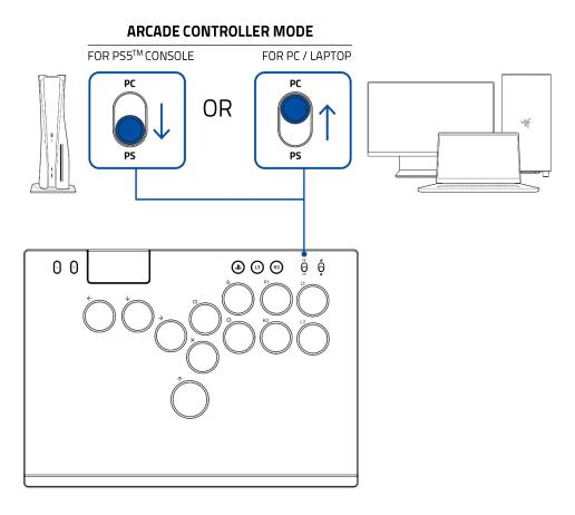
2. Plug the controller into the  $PS5^{TM}$  console or PC using the USB Type A to USB Type C cable.
